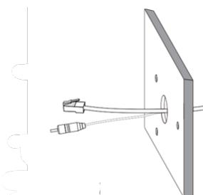
If using additional mounting hardware (a backbox or pendant cap and wall arm), prepare and mount the hardware to the surface.
